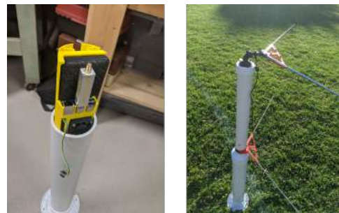
Figure 1: Left: showing the final packing of the Raspberry Pi, its battery, fan, and SDR into the PVC antenna stand. Right: The fully assembled set-up with a V-dipole antenna. 3D printed guides keep the antenna at 120 degrees.
