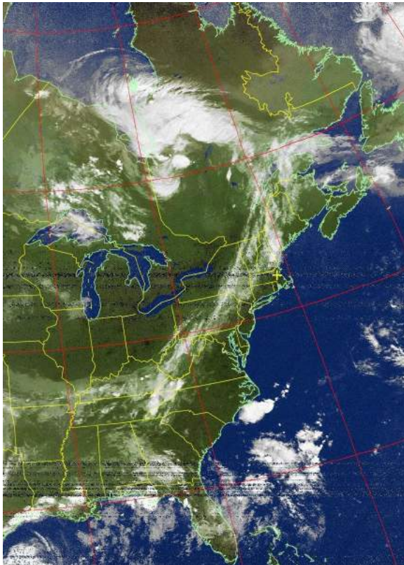
Figure 7: NOAA 18 northbound pass at 28 Jul 2020 14:58:09 GMT on 137.9125MHz, MCIR enhancement, Normal projection, Channel A: 2 (near infrared), Channel B: 4 (thermal infrared). Taken with a V dipole antenna. Maximum SNR for this picture was around 32dB.
