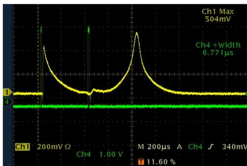
Figure 3: An oscilloscope screenshot showing both the applied pulses (green) and the resulting signal (yellow) in order to measure  $T_1$  for sample 2. The FID can be seen after the initial pulse, followed by the echo at a later time.
