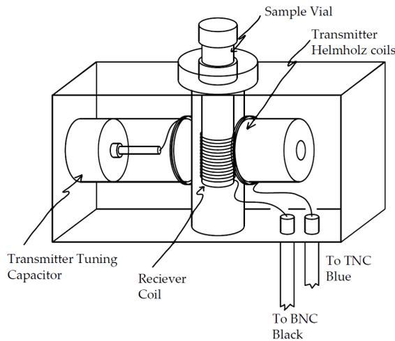
Figure 1: A diagram of the NMR, showing where the sample is placed, the transmitter Helmholtz coils where the oscillating magnetic field is applied, the receiver coils where the sample's signal is picked up, and the chamber where the sample is inserted [1]. In this diagram, the  $+\hat{z}$  direction is coming out of the page.
