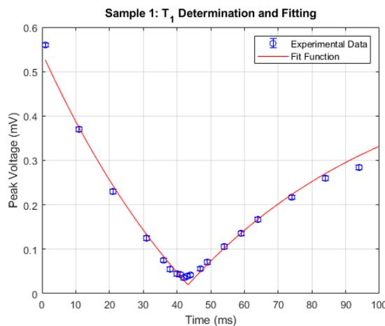
Figure 5: The data and fitting for  $T_1$  of sample 1.
