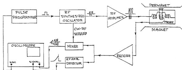
Figure 2: A block diagram of the provided TeachSpin apparatus [1].
