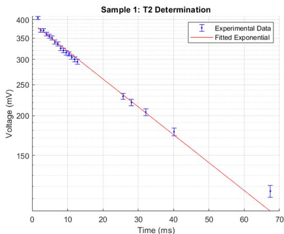
Figure 7: The data and fitting for  $T_2$  of sample 1.
