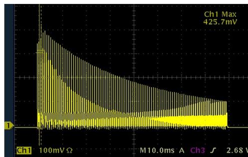
Figure 4: An oscilloscope screenshot showing the resulting signal (yellow) of a  $90^\circ$  pulse followed by many  $180^\circ$  pulses of alternating sign in order to measure  $T_2$ . The behavior of a decaying exponential can clearly be seen.
