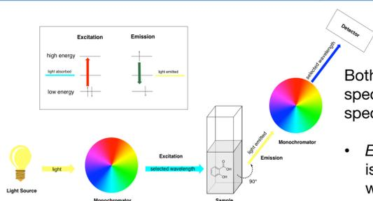
Both excitation and emission spectra can be measured in a spectrofluorometer.
