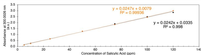
Figure 7: Using UV-vis spectroscopy, two calibration curves of salicylic acid in H<sub>2</sub>O (black) and a H<sub>2</sub>O/EtOH mixture (orange) were generated.
