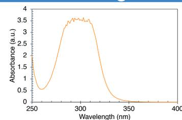
Figure 5: Oversaturated UV-vis scan of 240 ppm solution.
