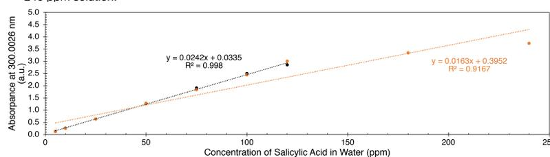
Figure 6: Using UV-vis spectroscopy, two calibration curves of salicylic acid in H<sub>2</sub>O (black) and a H<sub>2</sub>O/EtOH mixture (orange) were generated with a greater range of concentration.
