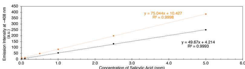
Figure 8: Using fluorescence spectroscopy, two calibration curves of salicylic acid in H<sub>2</sub>O (black) and a H<sub>2</sub>O/EtOH mixture (orange) were generated.
