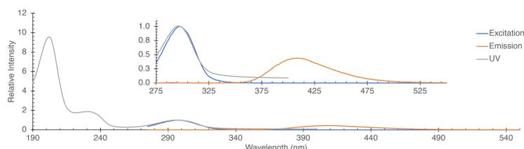
Figure 3. Using fluorescence spectroscopy, excitation (blue) and emission (orange) spectra of a Clear Pore® solution diluted with distilled water were taken, and an absorption scan (grey) was taken using UV-vis spectroscopy. The relative intensities of all spectra were scaled for comparison.
