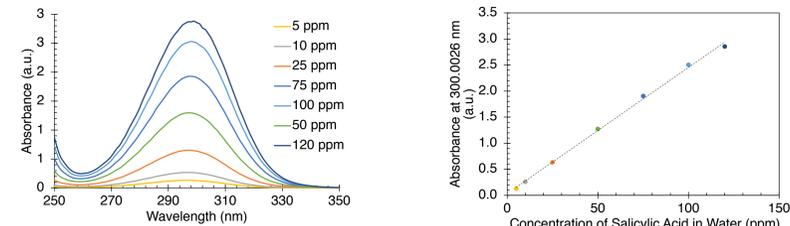
Figure 4: Calibration curves are developed from varying concentrations of salicylic acid and extracting the maximum absorbance or emission value from each spectrum (ex: 300 nm from the absorbance spectrum). Then, this maximum intensity value is plotted against the respective concentrations.
