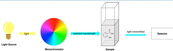
Figure 1. Ultraviolet-visible spectroscopy (aka UV-Vis) is an instrumentation method that determines absorbance of light by detecting transmitted light through a sample.
