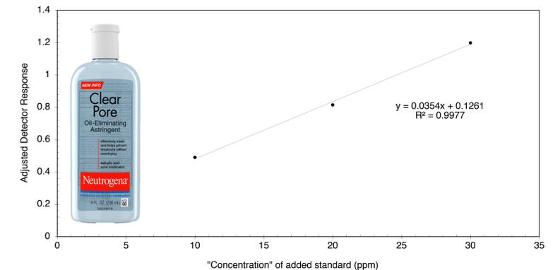
Figure 9: Using UV-vis spectroscopy, a standard addition curve using a diluted CP solution and a 100 ppm salicylic acid in H<sub>2</sub>O/EtOH standard was constructed. This was generated using the standard addition equation:
