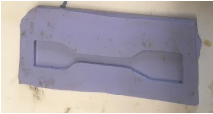
Figure 4: Mold used for the oak-water glass samples
