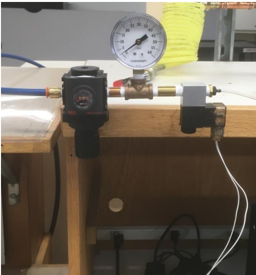
Figure 3: Left to Right: manual air pressure regulator, barometer, solenoid valve
