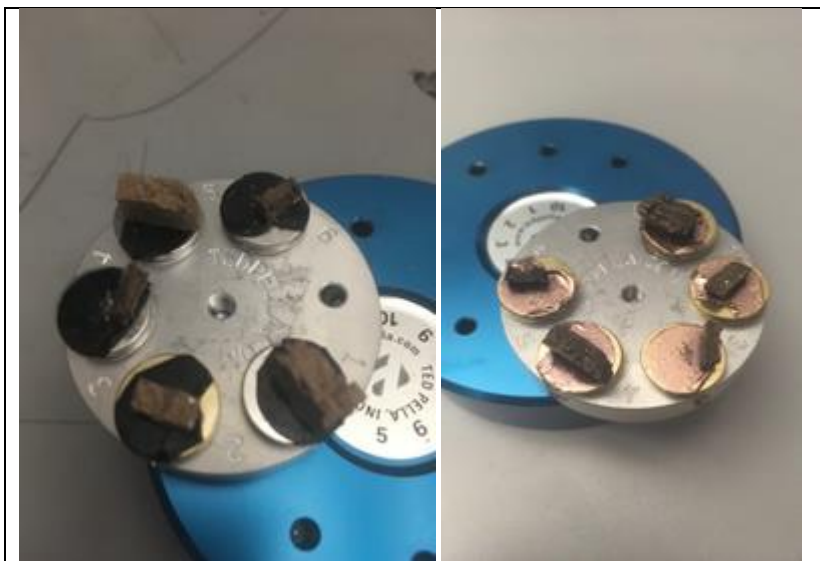
A before and after of the gold-coating process on our 5 samples
