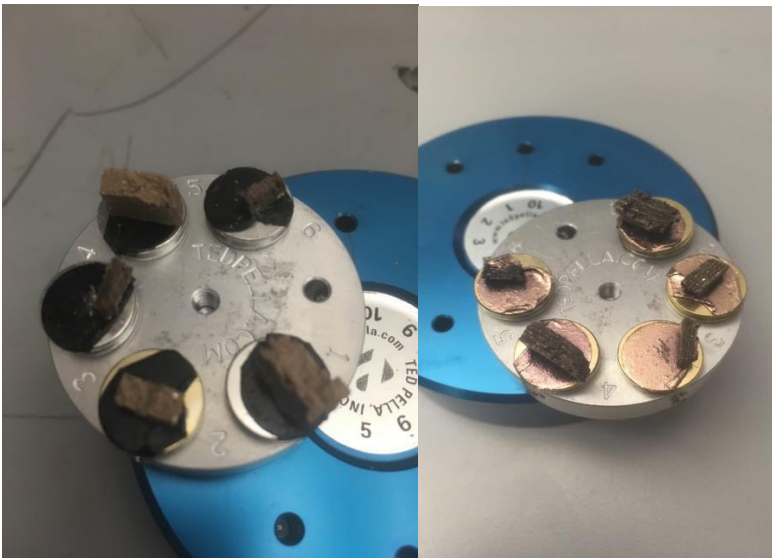
Figure 4: A before and after of the gold-coating process on our initial samples
